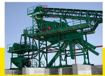
The pumping group consists of a hopper with a pyramidal trunk shape and a centrifugal pump, in which the watersand mixture to be treated comes from the installation. The pump drives the mixture to the hydrocyclone with the proper pressure and concentration. The purpose of the receiver hopper is to maintain a stable level of power to the pump, with a mechanical device.
